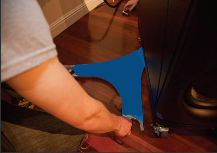
**STEP 2:** Slide the rear extension of the Q7 lift plate, padded side up, between the two rear casters. And then slide right side to the other side of the speaker.
