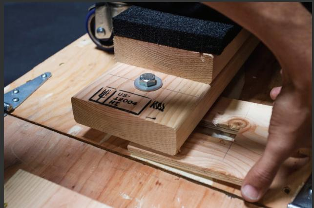
Using a  $\frac{3}{4}$ " socket wrench, turn the bolt at the base of the speaker clockwise until the 'C' shaped piece of wood can be slid out from underneath. With the wood removed turn the same bolt counter clockwise to lower the foam platform to the base of the crate.
