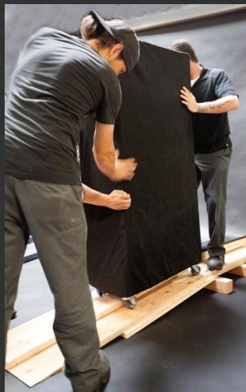
With one person behind the speaker and two in front, Push/pull the speaker towards the ramp. Apply pressure to the sides of the front of the speaker, careful not to touch the drivers, to ease the speaker straight down the ramp and onto the floor. Remove the crate.
