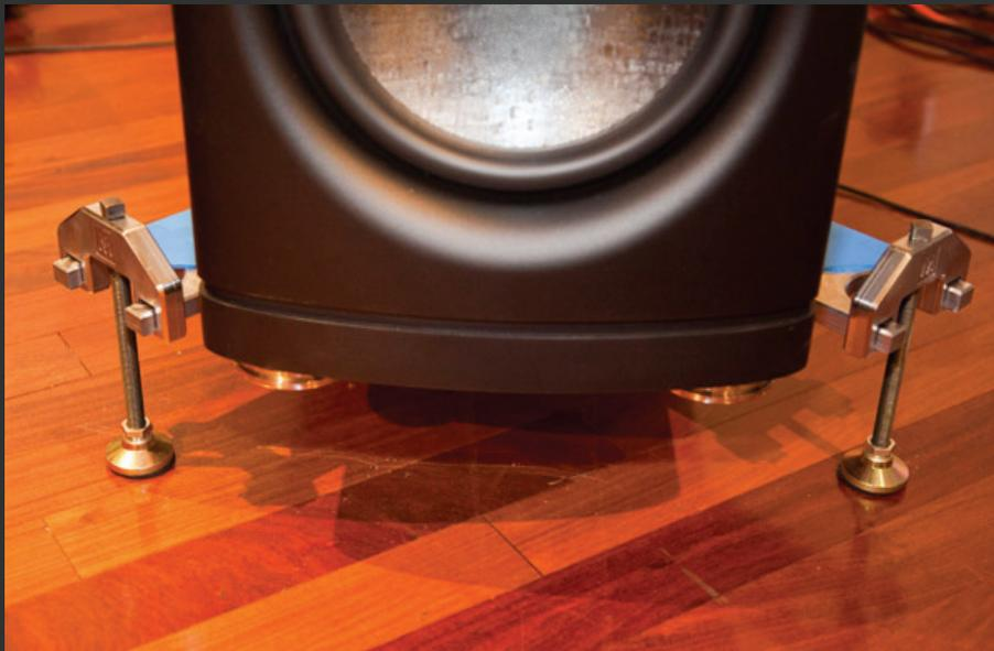
**STEP 6:** Once the Jacking bolt heads bottom out against the Q7 lift foot brackets, remove the caster and replace each with a Q7 foot assembly. Before the Q7 foot assemblies are installed, the two pieces should be separated so there is approximately 1/4" of space between the base and top piece. **NOTE:** This can be adjusted after the loud-speaker is lowered with the supplied spanners in the accessory kit.
