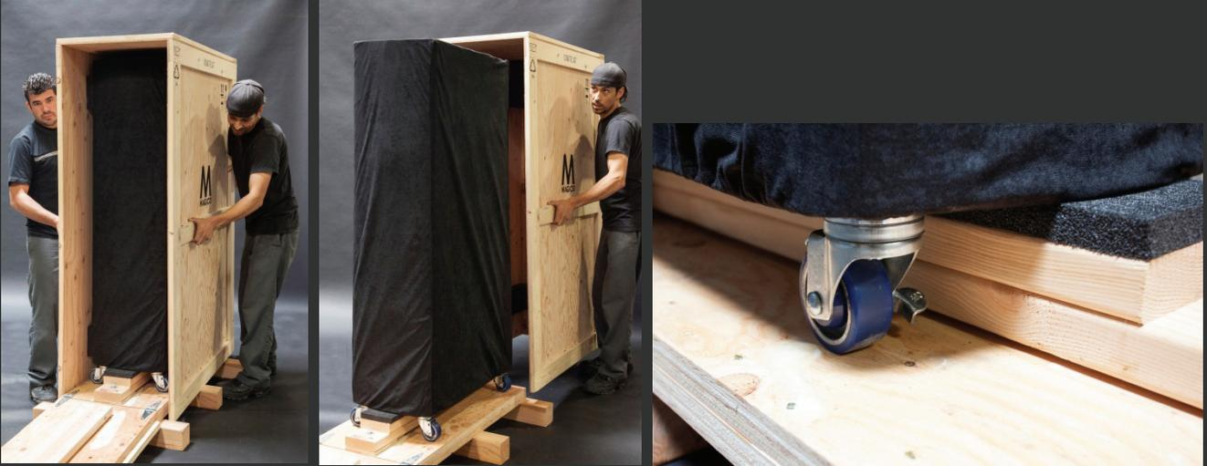
With one person on either side of the crate walls, lift straight up and backwards, removing the walls of the crate. Set walls aside. The speaker will be sitting free on the base. Disengage the brakes on the casters; position the casters parallel to the ramp and facing the back of the crate for smooth removal.
