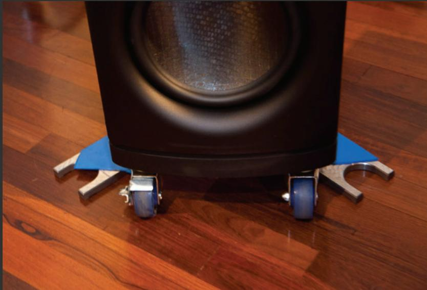
**STEP 3:** With one person at the front and back of the loud-speaker, work together to lift the Q7 lift plate from the ground so the padded material sits flush with the bottom
